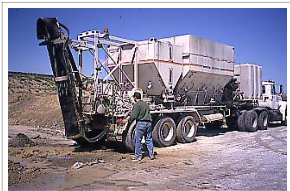
Figure 5-18: Volumetric mixer used for production of fast setting and excavatable CLSM in the Chicago area.
